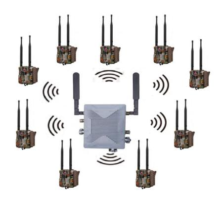
Base stations transmit data collected from the slave cameras to the control center via Internet/4G network/Optical fiber.
